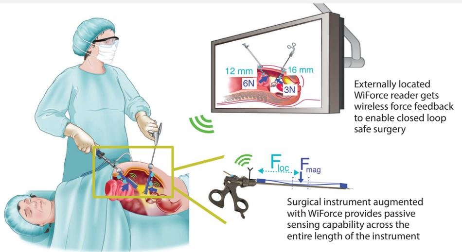
**FIGURE 2.** Passive wireless force sensing can help the surgeons perform safer minimally invasive surgeries, by feeding back the contact locations and force.
