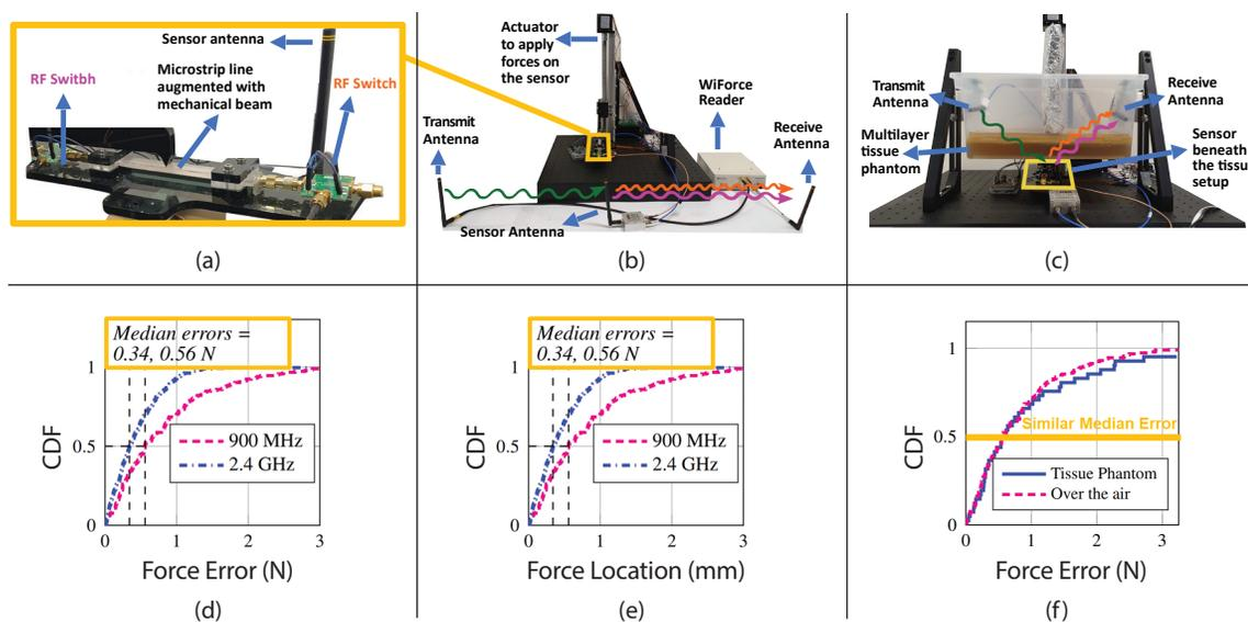
**FIGURE 4.** WiForce Experiment Setups and Benchmarking results: (a) WiForce Sensor Prototype. (b) Over the air evaluation platform. (c) Tissue phantom evaluation setup. (d) WiForce's force sensing performance. (e) WiForce's force localization performance (f) WiForce's robustness to in-body propagation.
